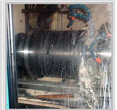
GPS240 during grinding
