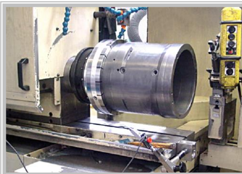
GPS240 with magnet and work piece
