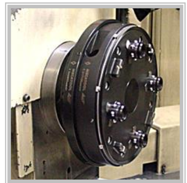
GPS240 built on spindle
