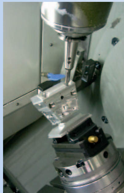
The second cell with the workpiece in a vice on the MacroMagnum pallet
