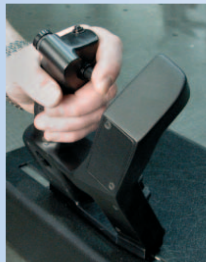
The simulated throttle control with 24 functions is highly responsive. Large movements must be avoided if the user is to retain fingertip control of the “equipment”
