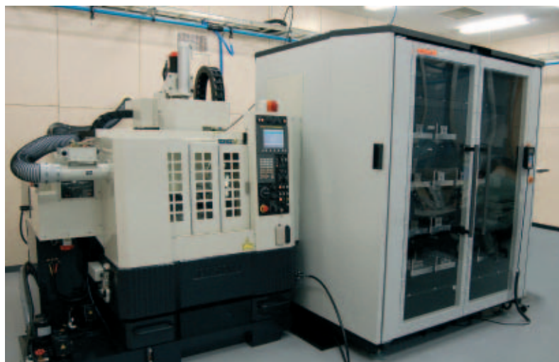
The supreme milling cell with WorkPartner and WorkShopManager
