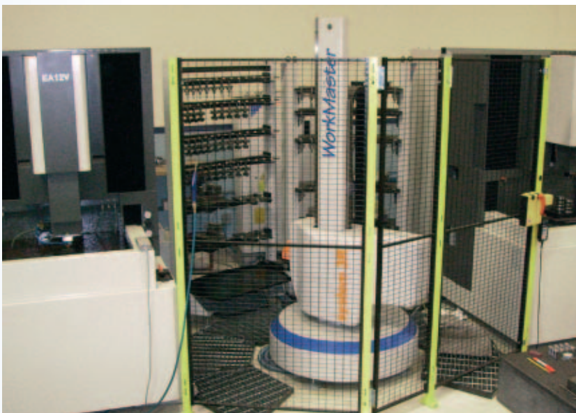
The magnificent double cell, two die-sinking EDM machines and a WorkMaster. The longest a single job has run here is 42 hours – unmanned!
