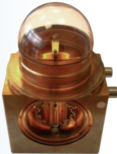
Copper components for radiation equipment; 3.5 hours of machining in four set-ups. Final weight, 4.5 kg.
