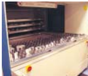
A tray of electrodes at the access station of the Lean-Lift is ready for transport and loading into the storage rack of a die-sink EDM cell
