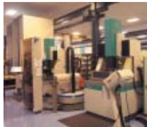
Dual "drop tank" Ingersoll die-sink EDM machines are working around-the-clock, while being loaded and unloaded by a WorkMaster
