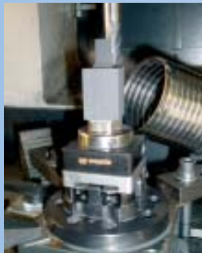
Milling graphite electrodes in MacroJunior holders
