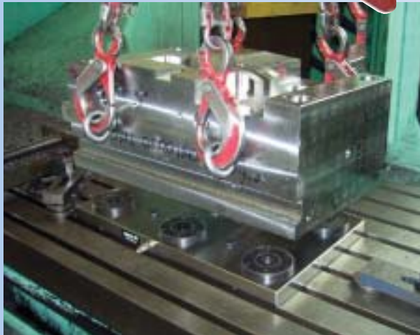
The Delphin system offers fast and precise set-up of mould bases in the milling machines.
