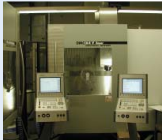
The magnificent double cell generates revenue during the dark hours. A DMU 50 evolution and a DMC 64 V Linear positioned at an angle to each other are served by a WorkMaster.
