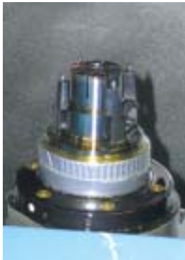
Mecatool palletisation at work in a milling machine.
