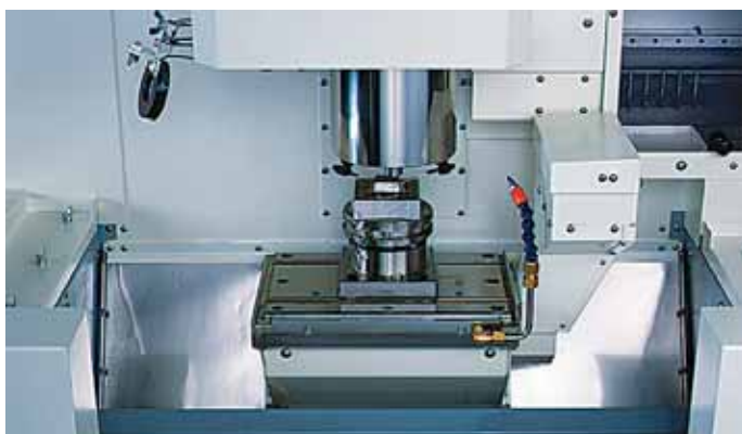
A micromold positioned in a referencing system is machined on a Makino Hyper 2J vertical machining center.
