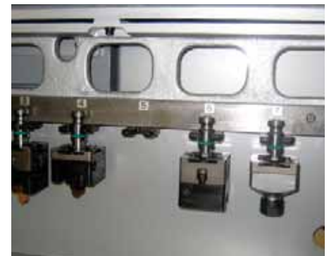
Electrodes are fitted to Macro holders in the die-sinker's toolchanger, which provide assured repeatable accuracy in the EDM process.
