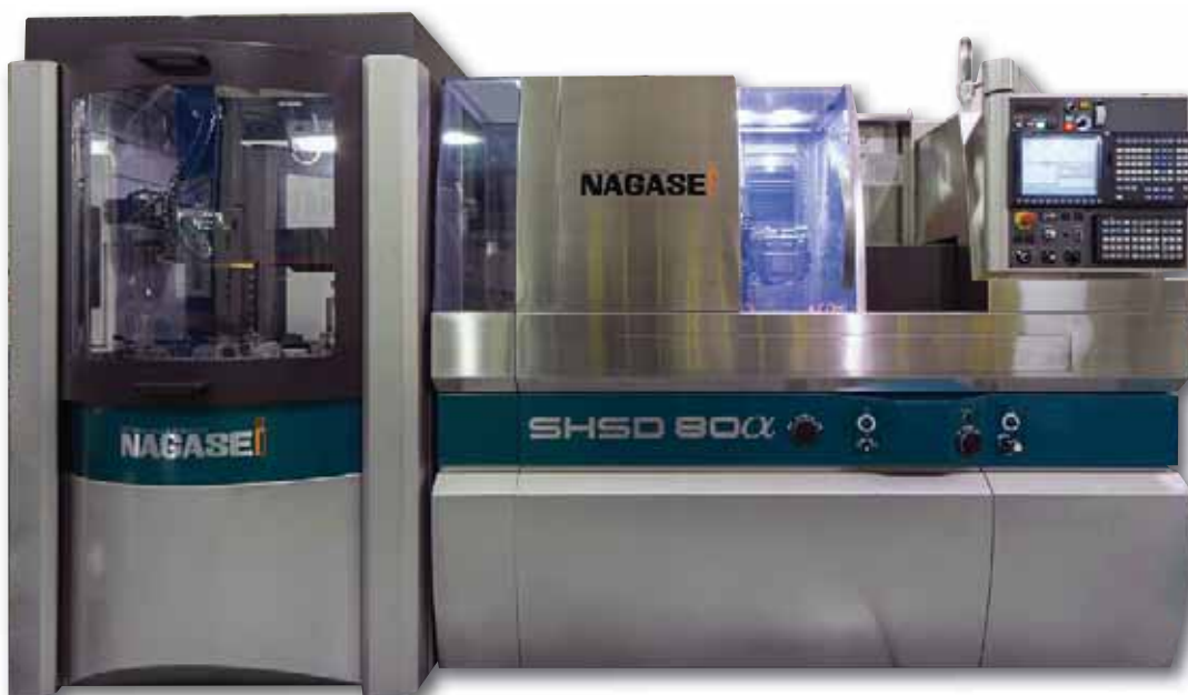
Production cell that the Japanese Chamber of Commerce and Industry awarded the "President's prize". On the left side "behind the cover" Automation solution from System 3R – WorkPal Compact Servo.
